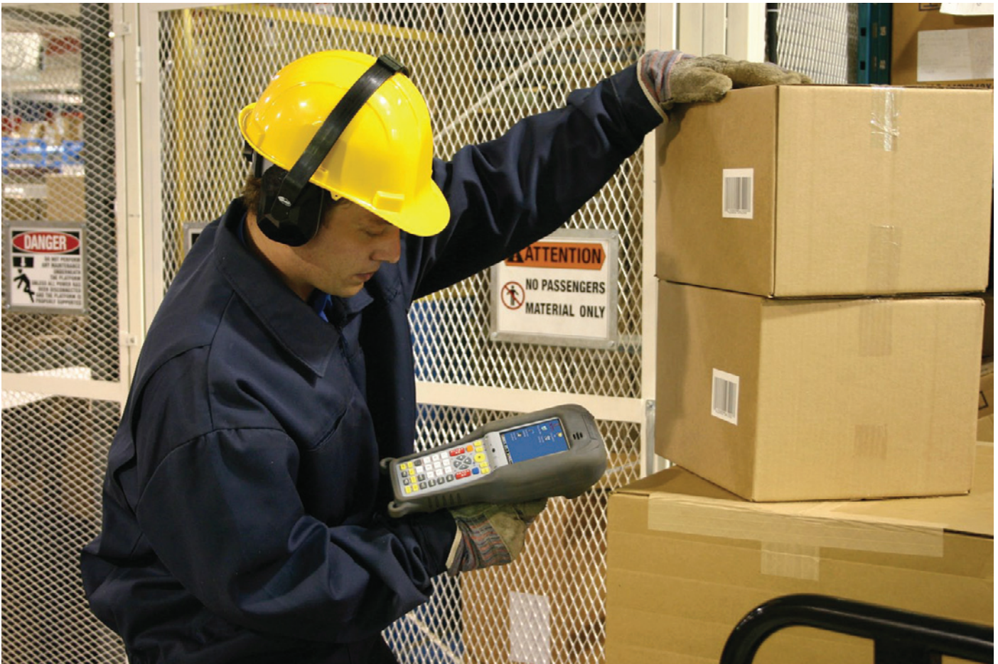
The 7530 offers advanced ruggedness with an IP67 rating against dust and water. Superior single-piece molded plastic construction and hard-cap keys provide durability to withstand 6' drops to polished concrete.
